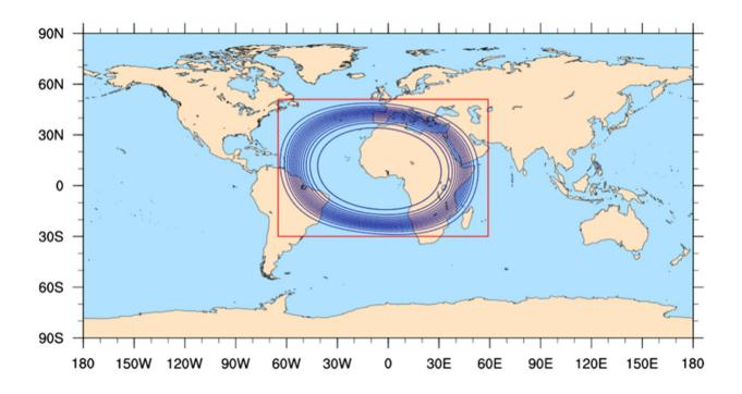
Illustration of the 15-km to 3-km variable resolution mesh and Limited-Area domain (red square) configuration produced using MPAS Tools (https://github.com/MPAS-Dev/MPAS-Tools). Contours are in  $1.6-7.2 \times 10^7$  km by  $0.4 \times 10^7$  km. Credit: *Journal of Advances in Modeling Earth Systems* (2024). DOI: 10.1029/2023MS004070
