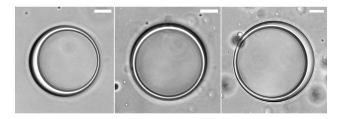
Differential interference contrast microscopy images show protein-RNA vesicles created in the lab. The vesicles -- hollow, spherical sacks -- were made without traditional lipid building blocks. The scale bar shows a length of 10 microns. Credit: Ibraheem Alshareedah
